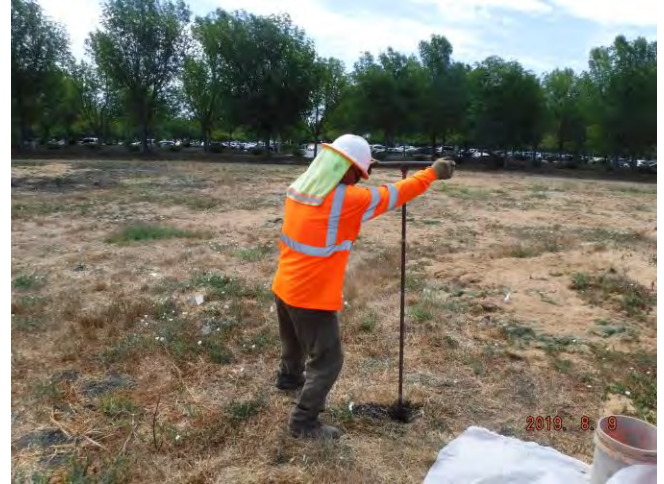
Photo 2: View of hand-augering.
